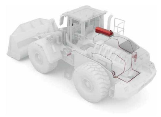
The Dafo detection system is designed to activate an alarm (sound and flashlight), adjust the vehicle operation (shutting down the cooling and ventilation fans as well as shutting down the fuel line to reduce the spread of fire) and activating the automatic fire suppression system.
