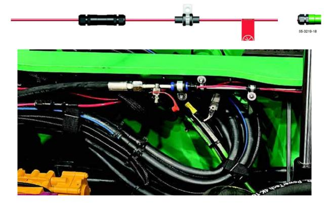
Large heavy-duty mining vehicles have large engine compartments. It is therefore important that the engine compartments are protected with additional suitable detection systems in addition to the linear heat detector which then provides the vehicle maximum fire protection.
