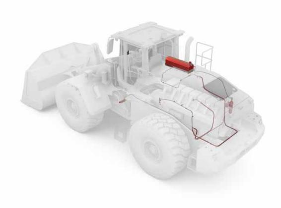
The Dafo Vehicle detection system is designed to activate an alarm (sound and flashlight), adjust the vehicle operation (shutting down the cooling and ventilation fans as well as shutting down the fuel line to reduce the spread of fire) and activating the automatic fire suppression system.
