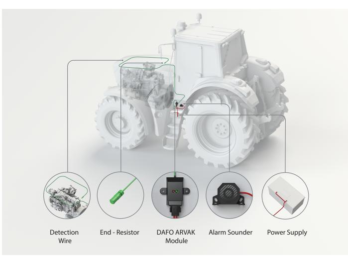
Arvak is a cost-effective, stand-alone safety device designed to provide early fire detection and advanced protection for high-risk areas. With its fast installation process and robust design, it ensures reliable performance without the need for annual servicing if used as a stand-alone system.
