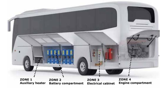
The different protection zones are then protected in various ways by robust detection and suppression systems – both liquid based and gas-based solutions.
